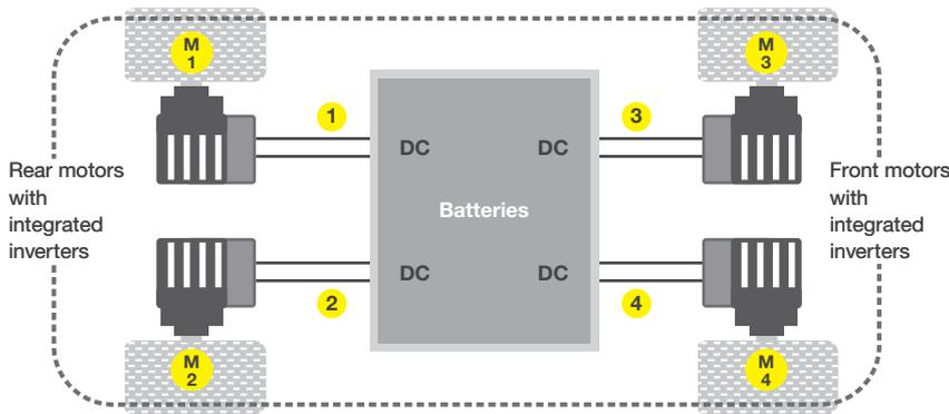
**Case1:** Modern drive systems with integrated inverters do not allow access to the AC signals. Here one of the main measurement tasks is to measure the overall drive train efficiency from DC to mechanical power. The example shows 4 DC measurements (1 to 4) with the corresponding 4 mechanical power measurements (M1 to M4)
