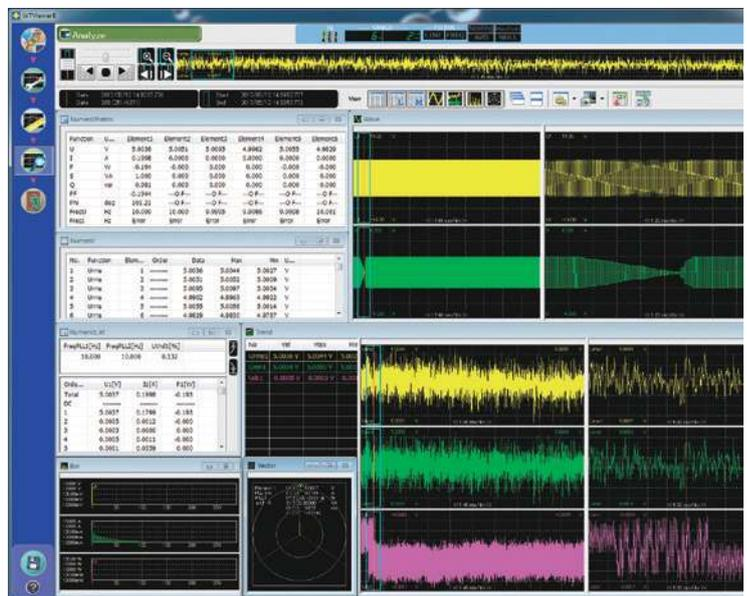
With customizable split screen display of readings in numeric, bar, trend or vector formats, the WTViewerE simplifies the acquisition, storage and analysis of multichannel measurements from up to 4 power analyzers simultaneously.
